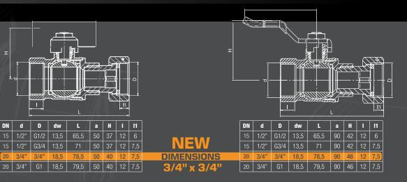
CUT-OFF VALVE WITH SWIVEL NUT
