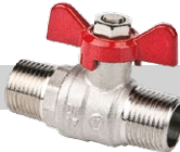
ONYX Nickel plated full-port ball valve with nut on stem and aluminium butterfly handle (male-male version)
